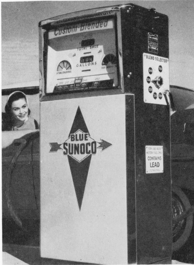
Left above:—This newly-developed gasoline pump, which dispenses six octane grades of motor fuel, is now operating at Sunoco service stations in Waterbury and surrounding areas.
